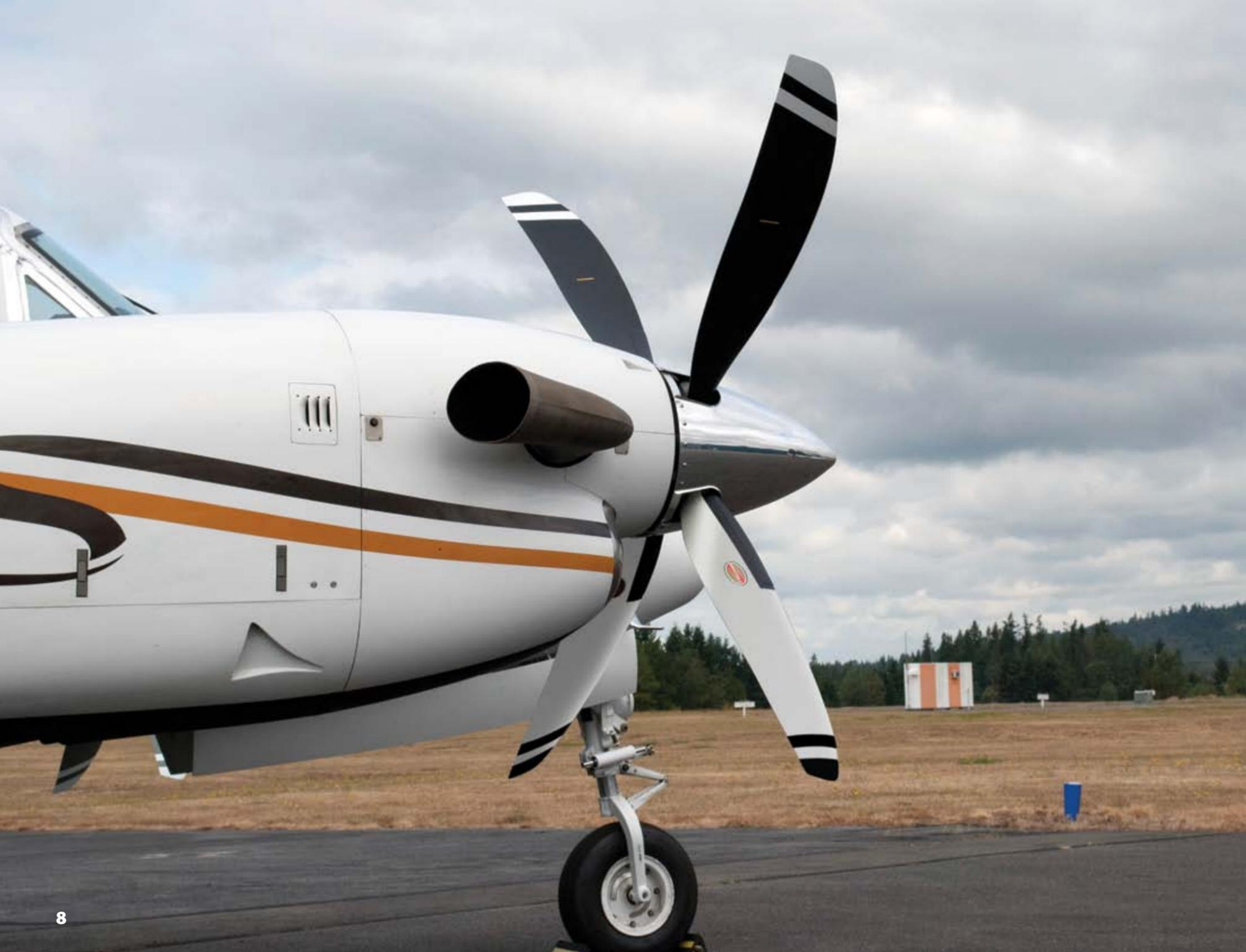
Introducing blade sweep to the blades can largely overcome these drawbacks. You are never going to get rid of noise, but blade sweep does allow you to increase diameter to increase performance without paying the normal penalties.
