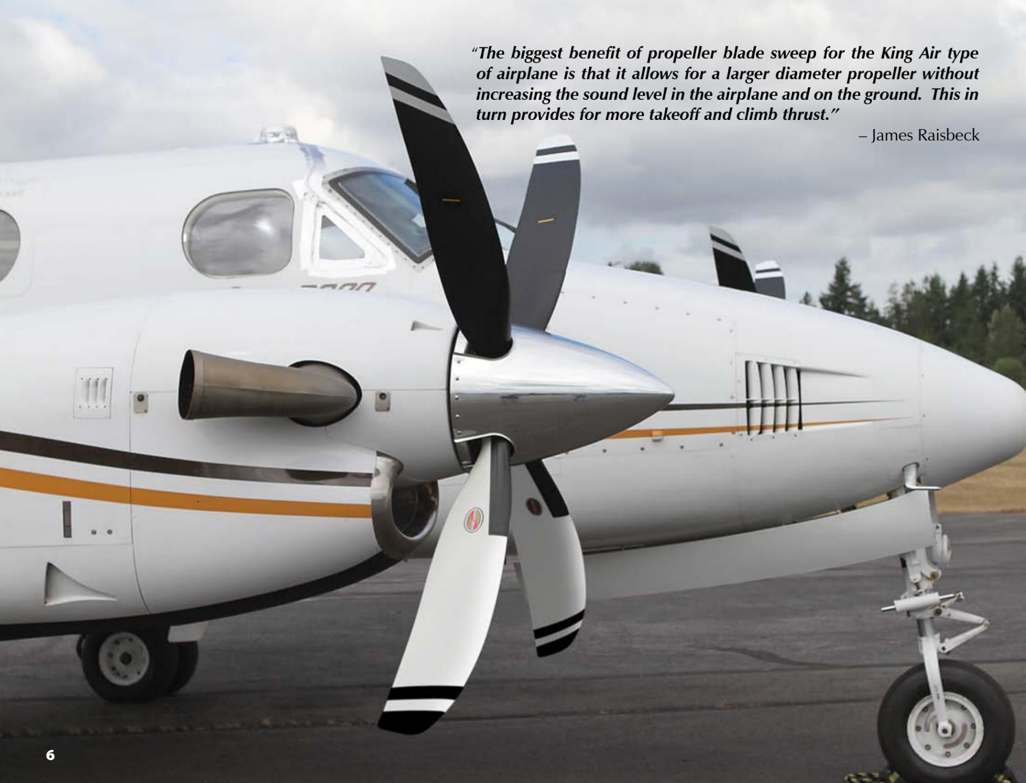
*“The biggest benefit of propeller blade sweep for the King Air type of airplane is that it allows for a larger diameter propeller without increasing the sound level in the airplane and on the ground. This in turn provides for more takeoff and climb thrust.”*
