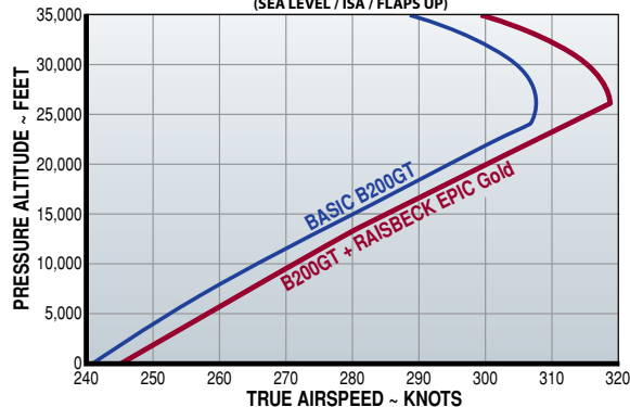
ALLOWABLE TAKEOFF WEIGHT COMPARISON RAISBECK EPIC B200GT vs BASIC B200GT (SEA LEVEL / ISA / FLAPS UP)
